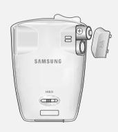
Insert batteries; paying attention to the orientation of the + and - ends of the batteries.
